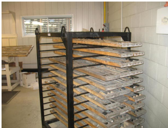
Core rack with selected witness core in thaw zone
