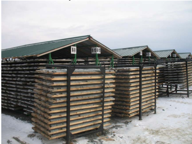
Figure 32: Permanent core racks and mobile core racks.
