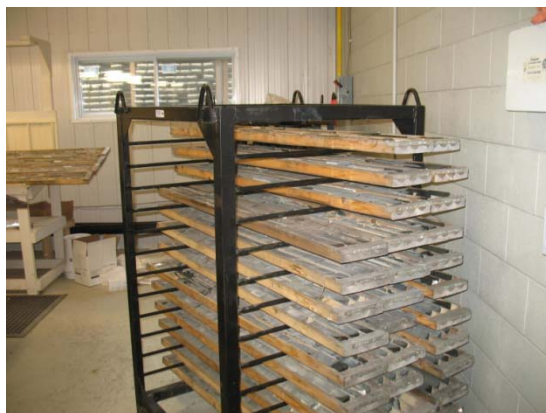
Core rack with selected witness core in thaw zone
