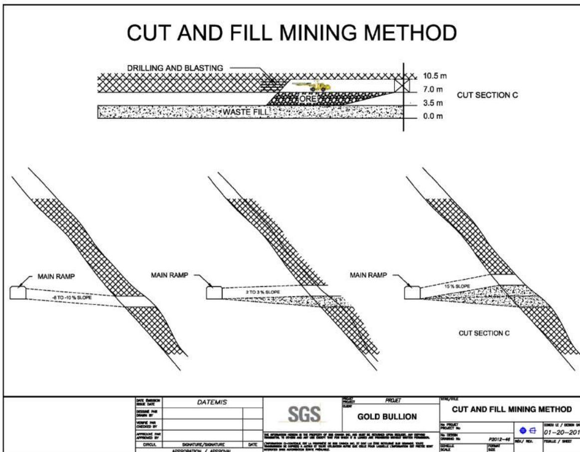
Figure 86: Drift-and-Fill method
