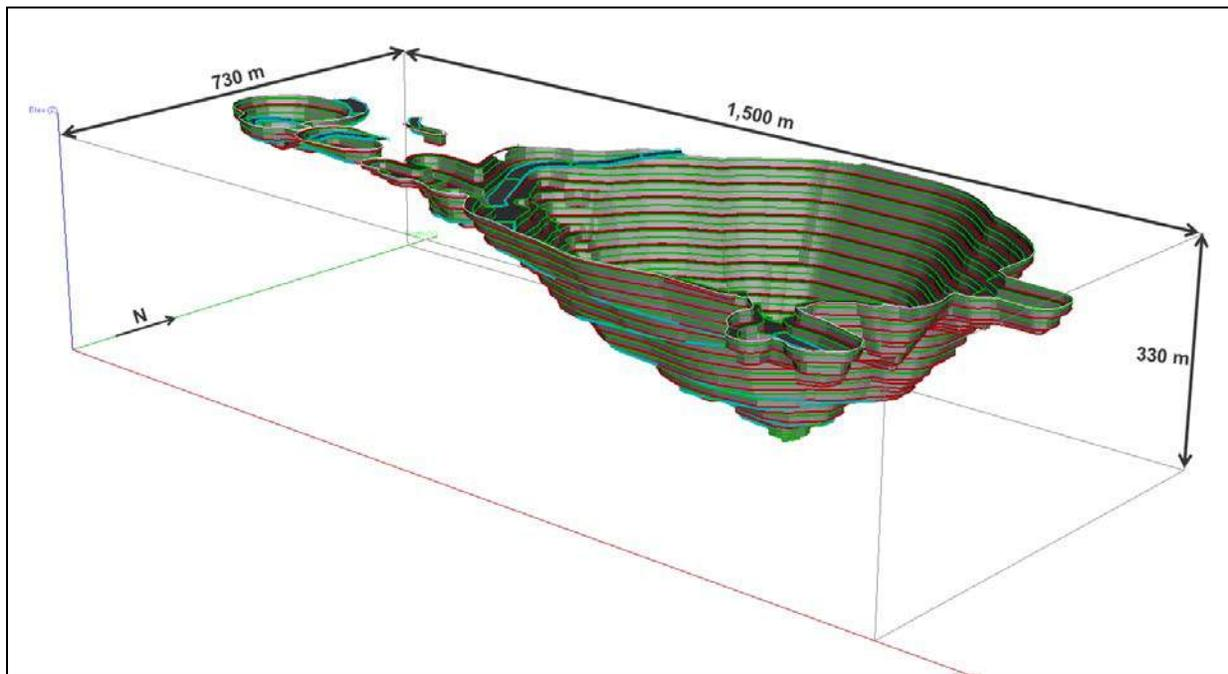
Figure 80: 3D view of the designed pit
