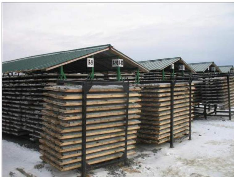
**Figure 32: Permanent core racks and mobile core racks**
