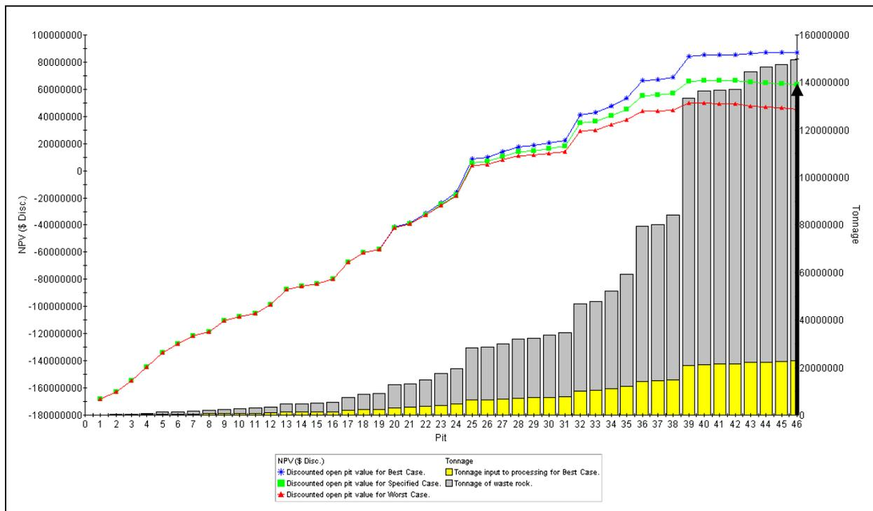
**Figure 75: Pit Tonnage versus NPV (\$) demonstrating optimal shell**
