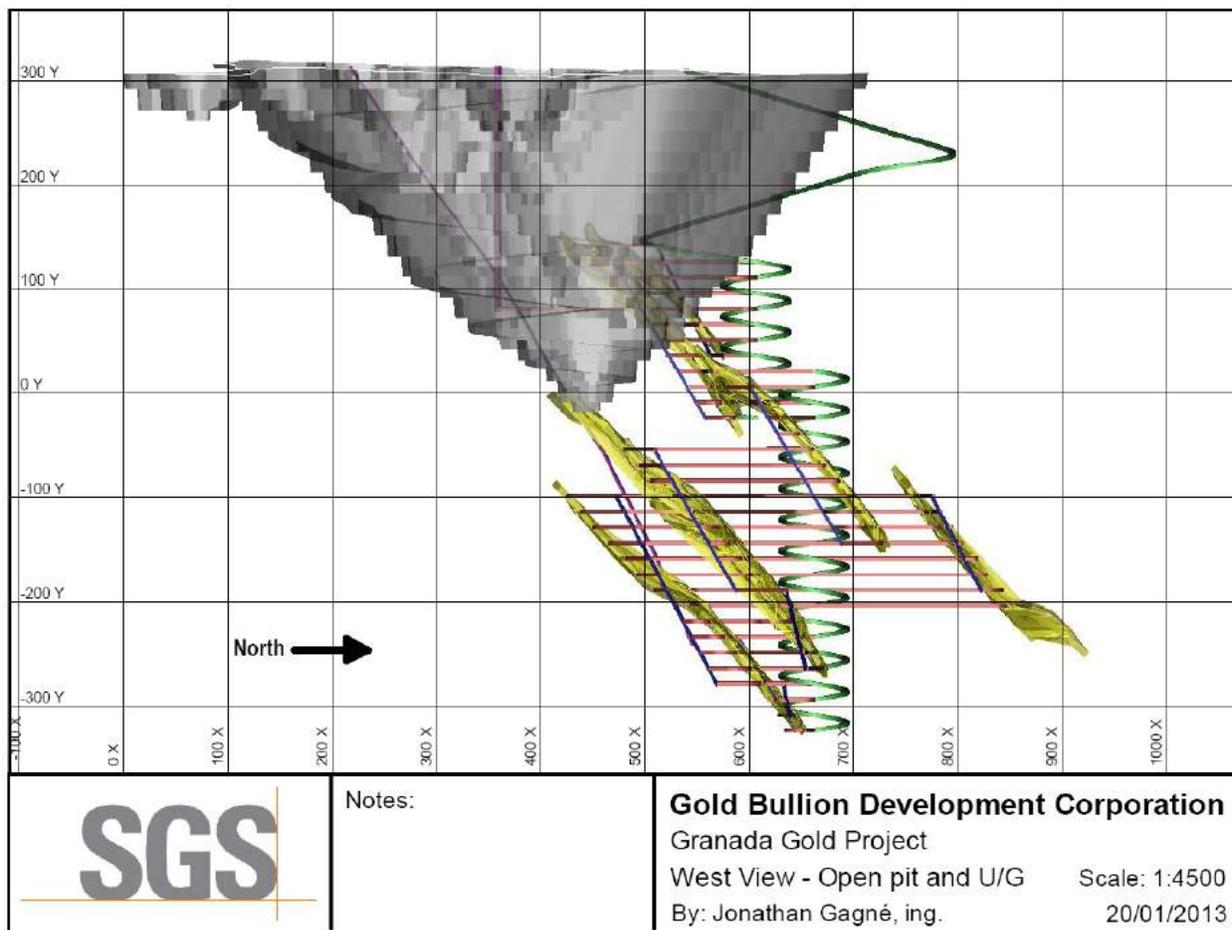
Figure 84: Open pit and U/G long section
