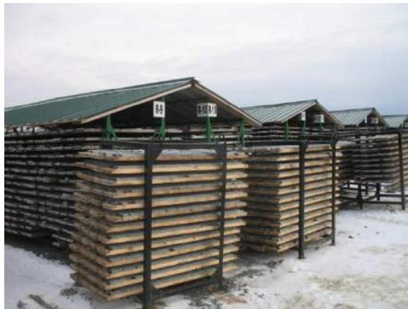
*Core boxes in racks and on steel carrier*
