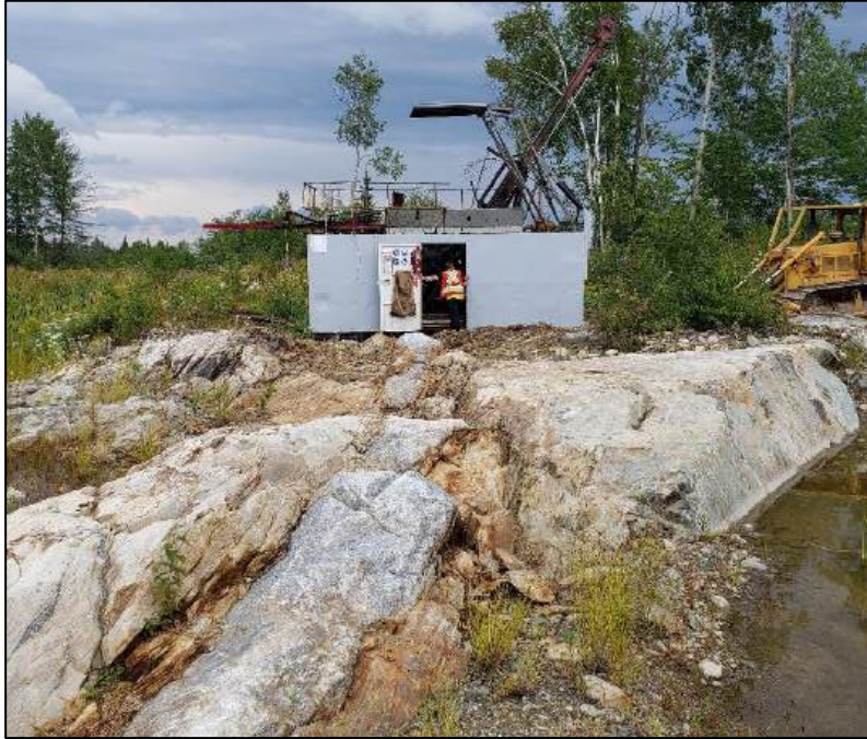
Figure 10-7 Diamond Drill on Quartz Vein at Granada Property
