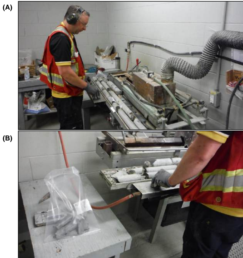
Figure 11-7 A) Core Samples cut in Half Using a Cutting Saw; B) Sample in Plastic Bag with Tag
