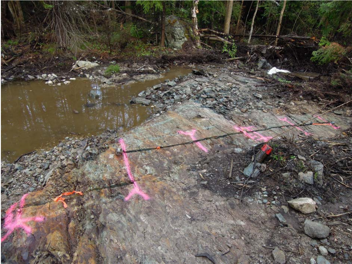
Figure 9-4: Channel sampling, 1 metre intervals TP-13-07
