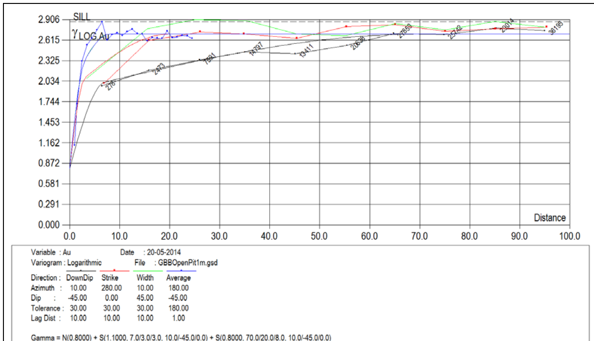
Figure 14-6: Variogram of 1 m Au composites Log capped at 30 g/t
