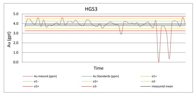
Figure 40: Standard Accurassay HGS3 Results for Au
