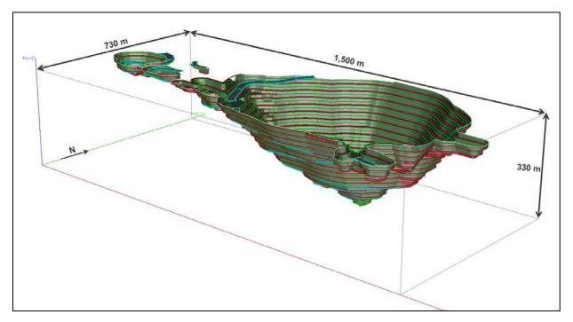
Figure 80: 3D view of the designed pit
