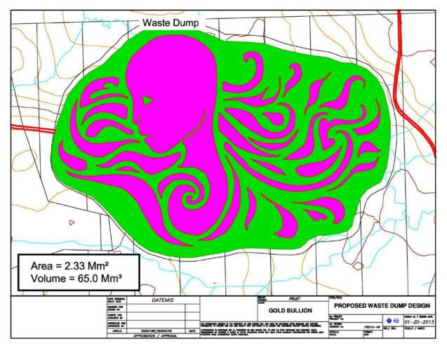
Figure 94: Waste Rock Stockpile Design
