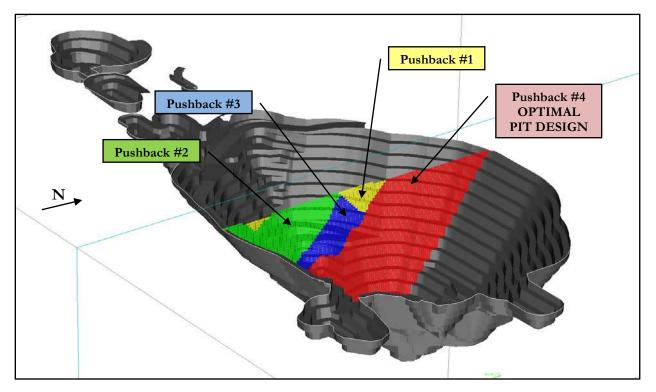
Figure 82: Typical section view of pushback's 1, 2, 3 and 4 (optimal pit design)
