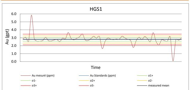
Figure 39: Standard Accurassay HGS1 Results for Au
