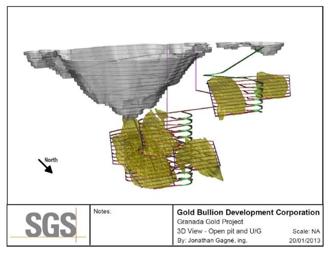
Figure 72: 3D View of Open Pit and Underground Mining
